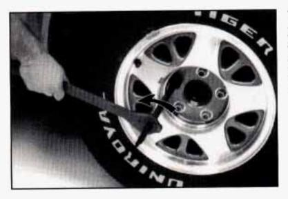
With DOWN facing you, use the ratchet and socket to loosen all the wheel nuts. Don't remove them yet.
